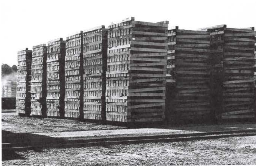
Figure 30-3-7. Broad View of a Clean, Well Drained Air-dry Yard Seasoning Ties
